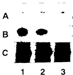
Fig. 2. Release of radioactivity from 32 P-labeled GAPDH. GAPDH was incubated with 50 mM Tris-HCl, pH 9.0, and 5 \mu M (185 kBq/nmol) [adenylate- 32 P]NAD + . The additions were none (A), 5 mM DTT and 50 \mu M SNP (B), and 5 mM DTT and 0.5 mM GA3P (C). The labeled GAPDHs were treated with 0.5 M NaCl (lane 1), 0.5 M NH 2 OH (lane 2), or 50 \mu M HgCl 2 (lane 3), and then analyzed as described under "EXPERIMENTAL PROCEDURES."
